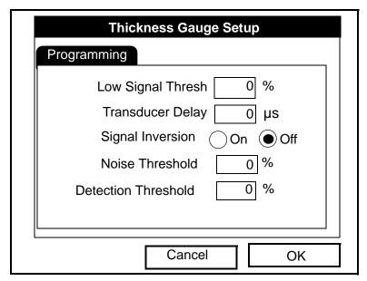
Figure 9-12: The Thickness Gauge Programming Window
